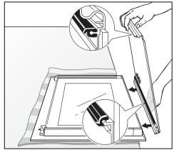
■ When replacing the inner pane make sure that the aluminium guide and handle face upwards. The words "Miele CleanGlas" will then be legible.
